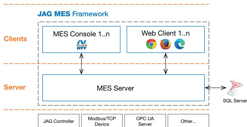
JAG MES has a classical Client / Server architecture designed for multiuser environments. The core of the MES Framework is the **MES Server**. It runs as a service and offers a large number of interfaces. For the graphical user interfaces it provides the backend to the MES Consoles (rich clients) and Web Clients. At the same time it interacts with the JAG and third party automation components on a PCS level and stores all data in SQL Server databases.
